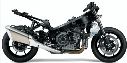
Mounted to new seven-spoke wheels are bigger 320mm discs up front, with improved stopping power also coming from Brembo Stylema calipers. Longer journeys on the new Hayabusa are not only made easier thanks to the extensive electronics package, but changes to the bike's ergonomics see the 'bars brought closer to the rider by 12mm, aiding rider comfort while ensuring the rider remains directly connected to the front wheels
