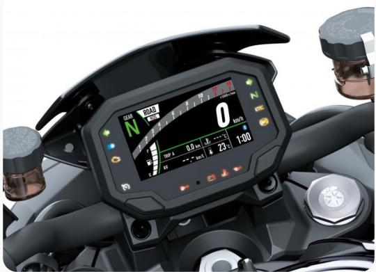
The instrument panel comprehensively displays various information on the full-colour TFT LCD screen. It also has functions that can help you manage daily vehicle operating status and schedule for long distance riding. Display functions include a digital speedometer, gear position indicator, shift indicator, odometer, dual trip meters, fuel gauge, remaining range, current/average fuel consumption, outside temperature, coolant temperature, clock, Economical Riding Indicator, IMU indicator, KIBS in
